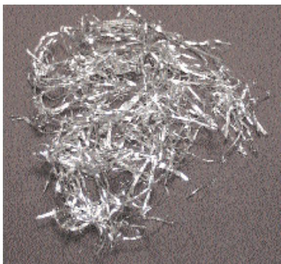
Fig. 2: Metallic ribbon obtained by melt spinning.
